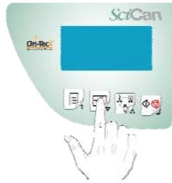
To select the **VACUUM TEST** program, press the **Test Selection** key one or two times until the display reads:
