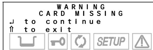
Ensure the data logger is properly connected and the proper memory card is installed then press the key ↓ on the command panel.
