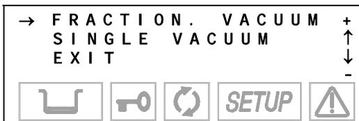
Select **FRACTION** to perform a fractionated vacuum (for hollow bodies and porous materials), or **SINGLE** for a single preliminary vacuum phase (for solid instruments). Move using the **+** and **-** keys and confirm with the **↵** key.
