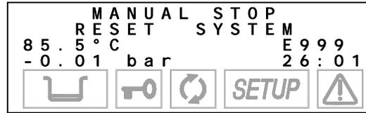
To **RESET** the system, press and hold the **PROGRAM SELECTION** key for at least three seconds until you hear the confirmation beep.
