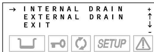
Selecting **INTERNAL DRAIN** enables the reading of the MAX level sensor in the internal tank. This is the setting that should be selected if connected directly to the drain.
