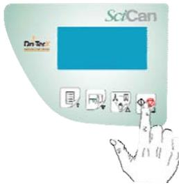
After placing the load in the sterilization chamber, select the desired program and close the door until you hear the click.
