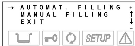
When **AUTOMATIC FILL** is selected, the unit will automatically fill the internal tank until the maximum level (MAX signal) is reached and the MAX icon is displayed.
