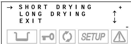
Select **LONG** drying for porous and/or wrapped loads, or **SHORT** if you need to sterilize solid, loose materials (and even hollow, as long as it is not wrapped). Move with the **+** and **-**, confirm with the **↵** key.
