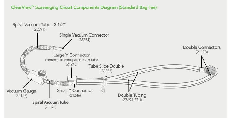
Note: For ClearView Scavenging Circuits for RFS and Accu-Vac, parts 25591, 22122, and 25592 are replaced with a  $6^\prime$  Spiral Vacuum Tube (part 27132)
