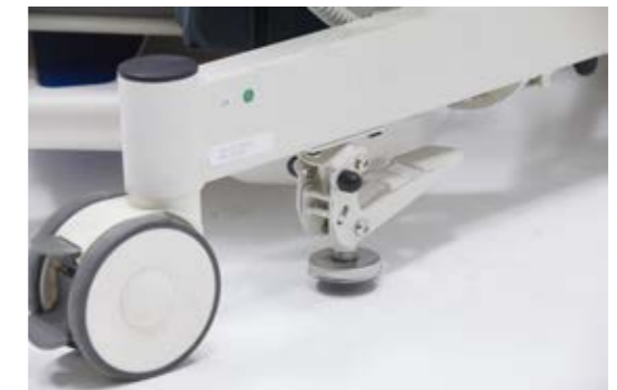
When the ground brake is released, the front wheel is stressed.
